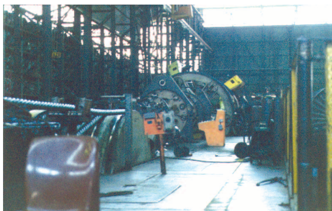
A length of rope being manufactured – usually in lengths of 1000m
